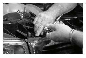
There are 2 bolts at the top of the grill assembly and 1 bolt in each of the turn of the turn signal openings. Using a 10mm socket remove all bolts. The grill assembly is still attached to the front by a few plastic clips at the bottom of the grill assembly. Place hands low and apart on the grill and pull straight out away from the van. Clips should pull free from front of van, set aside for later re-installation.
