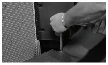
\*During this step have help as the bumper will free from the van once the bolts are removed.
