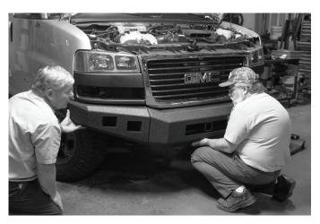
Tighten all bumper bolts after alignment is complete.
