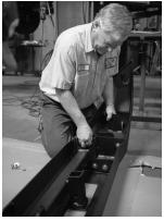
Install the center bumper skin over the steel bumper support frame. Using (6) 7/16" x 1.5" bolts/nuts/lock washers and (12) 7/16" flat washers to attach the skin to the frame. Snug but do not tighten these bolts as some adjustment may be needed later. Attach bumper wing sections to the center section using (6) 7/16" x 1.5" bolts/nuts/lock washers and (12) 7/16" flat washers. Again, snug but do not tighten the bolts for later adjustment.
