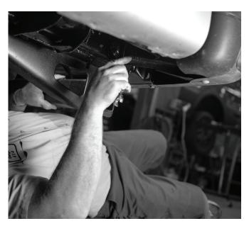
On the outside of the frame rails are bumper support mounts. Using a 15mm socket remove the 2 nuts holding the bracket to the mount and remove the bolt plate from the holes.
