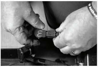
Insert each sensor into the mount making sure the white silicone ring around the sensor goes into the mounting hole without folding over. Attach the wiring harness to the mounts using cable ties provided.
