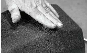
Place the wiring harness into the new bumper as it was placed in the old bumper. The main connector should be on the driver's side of the bumper. Locate each sensor plug at the sensor and connect to the sensor. Remember to push the red locking tab once the plug is securely attached to the sensor.
