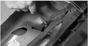
Once all the senors are removed from their mounts disconnect the wiring connector from each sensor. Make a note of each sensors location when removing as they will need to be installed in the same location on the new bumper. The connector for the sensor has a red locking tab that must be released first. Then press down on the small black connector tab to release the connector from the sensor.
